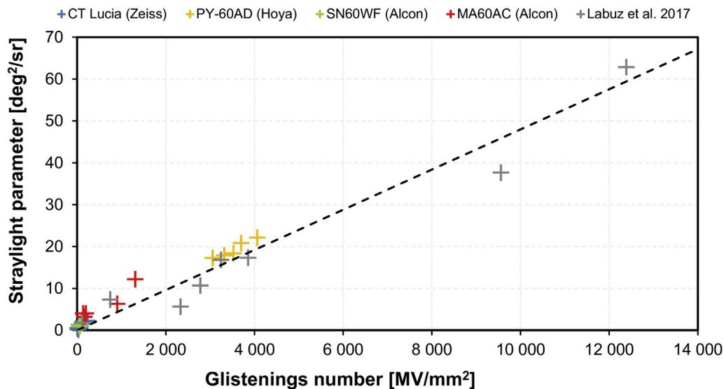
FIGURE 5. A proportional relationship between the straylight parameter and the glistening number in different lens models.
