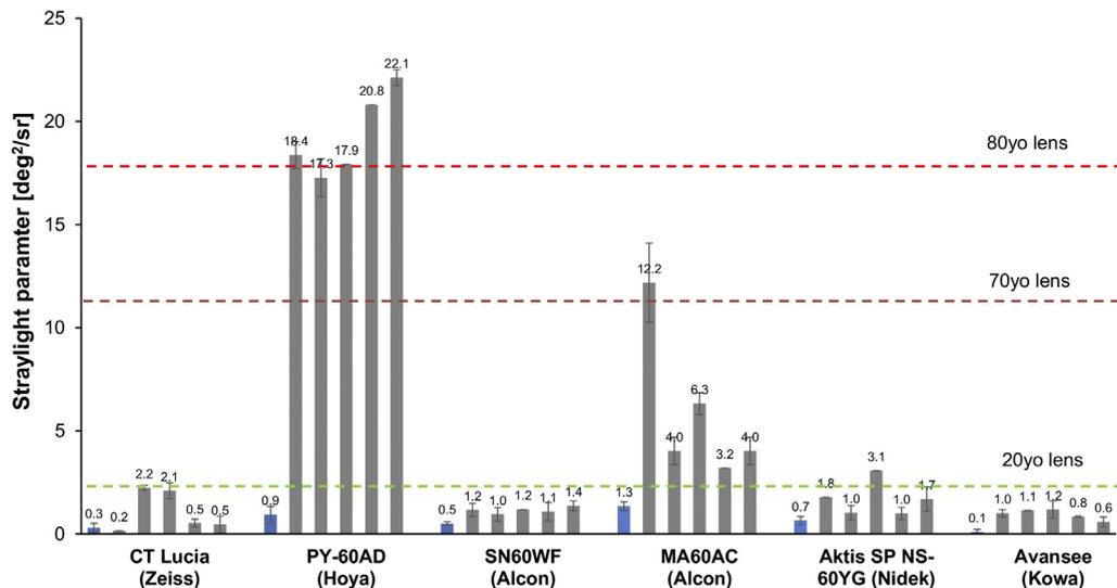
FIGURE 4. Mean straylight parameter across the studied intraocular lens (IOL) groups. The blue bars indicate straylight before IOL aging (control IOLs). The gray bars show straylight values of lenses after the aging procedure. The green line refers to a straylight level of a 20-year-old crystalline lens. The brown and red lines indicate straylight of the crystalline lens of age 70 and 80 years, respectively. Error bars = standard deviation.
