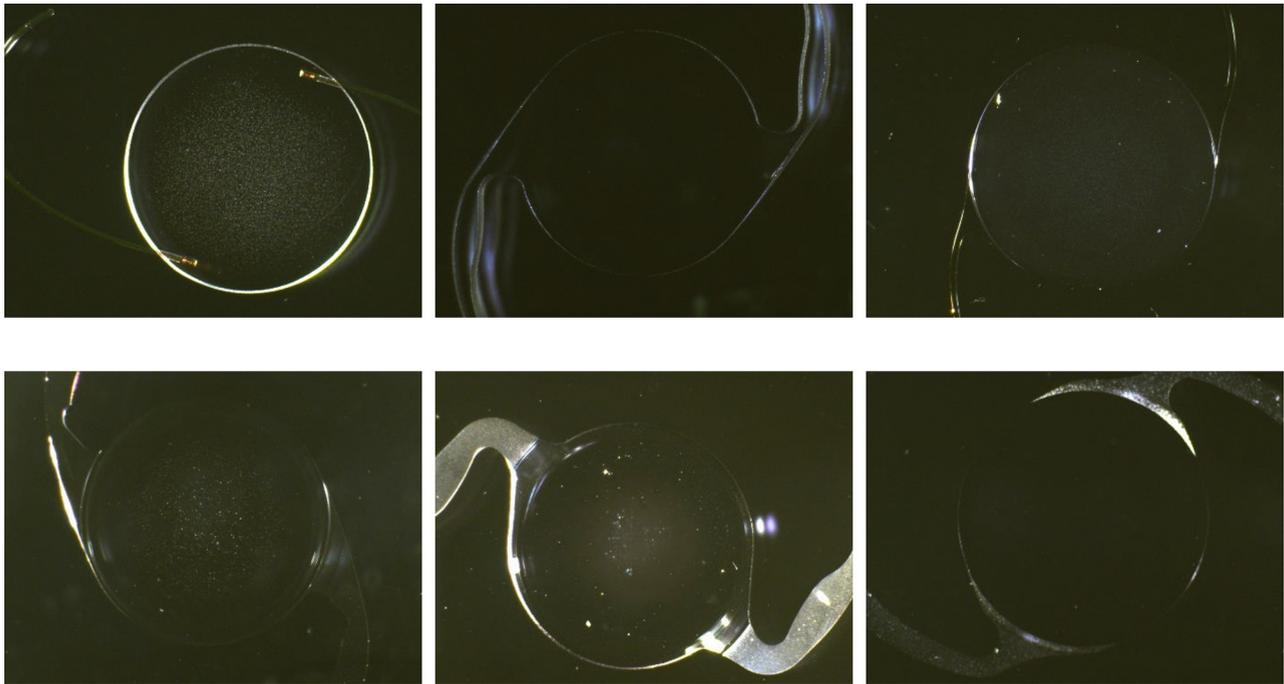
FIGURE 1. Microscopic images of the intraocular lenses after glistenings induction. (Top left) MA60AC (Alcon, Inc), (Top middle) SN60WF (Alcon Inc); (Top right) PY60AD (Hoya Surgical Optics), (Bottom left) CT Lucia 601P (Carl Zeiss Meditec), (Bottom middle) Aktis SP NS-60YG (Nidek), (Bottom right) Avanse (Kowa).
