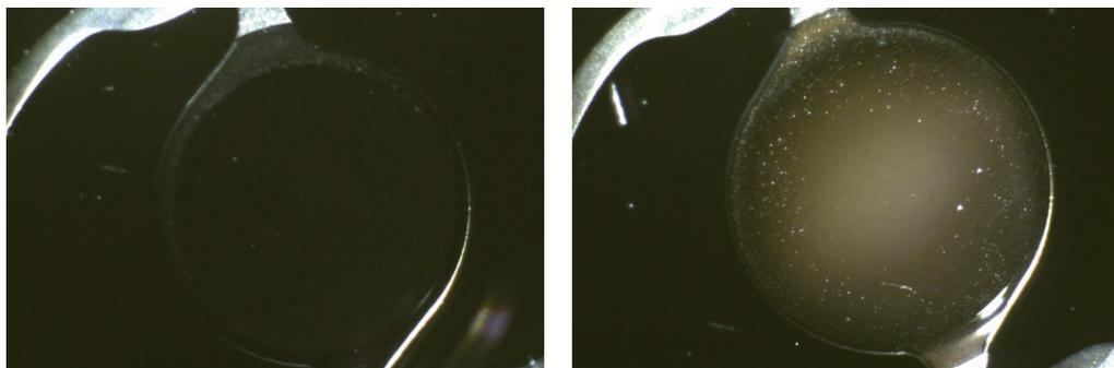
FIGURE 3. Photographs of an Aktis SP NS-60YG (Nidek) before (Left) and after (Right) the aging procedure. Note a white discoloration of the intraocular lens following aging.
